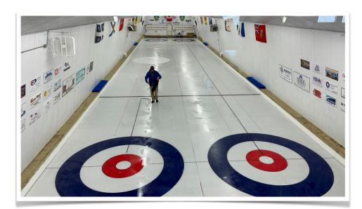
When curling stops, there are still 3-4 weeks of work for our Ice Techs! A majority of the lines that run the length of the ice are just ribbon. These get laid and removed individually. Once the ice is all removed the sheets get hung up to dry from the ceiling to get all the moisture out to ensure they are put away as dry as can be to ensure a long lifespan which saves the club money.
